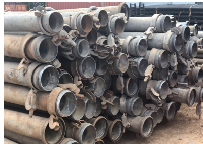
QD Piping, HDPE Piping, Hoses, & Fittings
